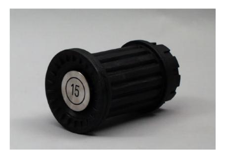
Freja nozzles is specially designed for Balder monitors or any other monitor with  $2\frac{1}{2}$ " water outlet. The nozzles are suitable for water and foam solutions. They are manufactured in a plastic composite with similar strength to aluminium.
